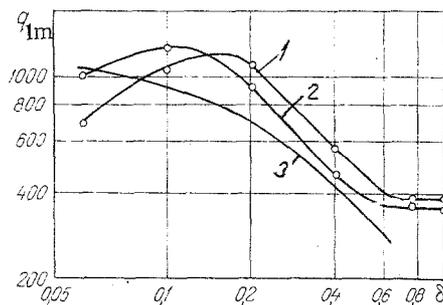
Fig. 4. Dependence of limiting heat flux ( $\text{kW/m}^2$ ) in the evaporation of water from a composite wick on the size of the gap (mm) between the screen and the heating surface: 1, 2) perforated screen,  $\alpha = 0.3$  mm,  $P = 0.5$  ( $p = 0.1$  and  $0.4$  MPa, respectively); 3) brass grid No. 056 under GOST 3584-73,  $p = 0.4$  MPa.
