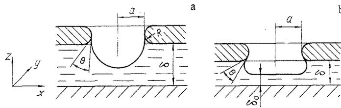
Fig. 1. Profile of the meniscus formed in a pore of a composite wick with different-size gaps  $\delta$ .
